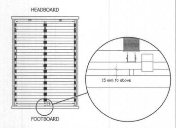
Adjust the bed base, make sure distance with the front footboard approximately 15mm to above gap as shown.
