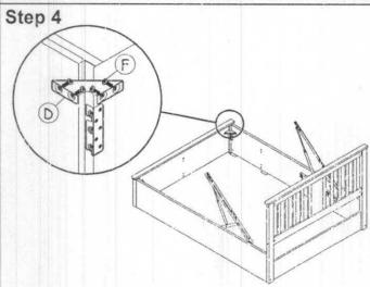
Fix metal corner block 'D' to the edge of footboard and side rails with bolts 'F' as shown.
