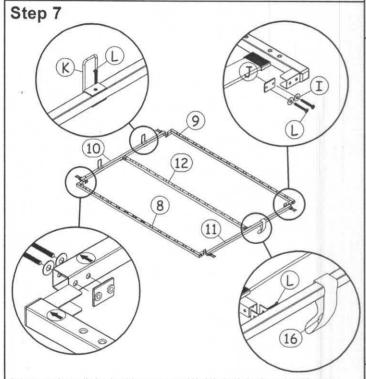
Join together all the bed base parts (8),(9),(10),(11) and (12) using hardware parts L. Attach hardware parts K using hardware part L and than attach hardware part 16 by slot to the part (11) as shown. Important note: Please assemble follow arrow direction.
