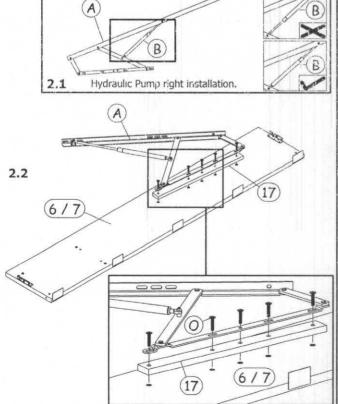
Firstly, fix the hydraulic pump to each hydraulic base as shown in diagram 2.1. Next, fix the left & right hydraulic spacer together with hydraulic base suppoter to the both side rails using bolts ' in diagram 2.2 and tighten all bolts.
