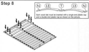
Place wood slats with plastic caps as above drawing. Then, fix it on the bed base by pressing it accordingly to the default holes. Ensure the plastic cap's pin is aimed to the hole.
