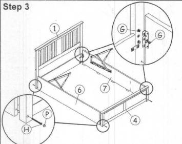
Fix side rails to the headboard and footboard with hardware as shown.
